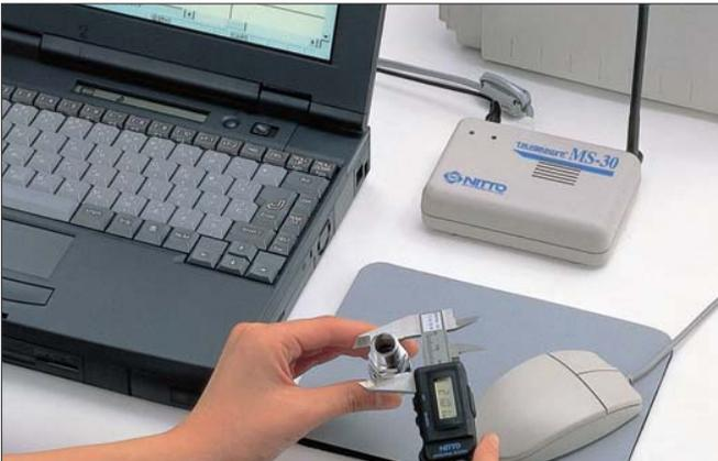
▲ Radio system enters and monitors measurement data
